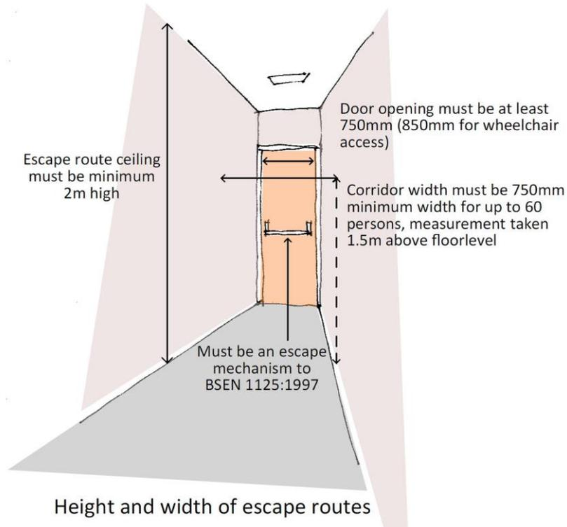
Building Regulations require the following minimum widths:
