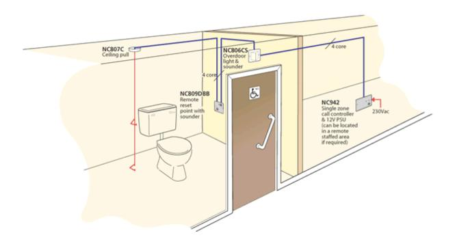
The single zone call controller is usually located in the corridor outside the WC, adjacent to the WC door, or it can be in a suitable remote area, such as an office, provided that area is always staffed when the building is in use, otherwise the alarm may not be heard.
